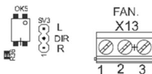
This jumper is used to set the correct turning direction of the stepper motor.
