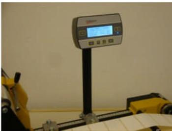
The port X103 is used to connect an external operator panel (in place of the original “potentiometer operator panel”) to the labeler.
