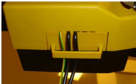
Special case **C4300-BUDGET**: the label scanner for this type of labeler will be connected directly to the main terminals on the main board (bottom). The label scanner cables are guided through the modular rail to the main board (entry of modular rail).
